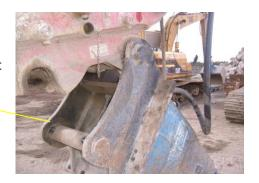
3. Ram Pushes a set of Jaws around the Pin of the Attachment
