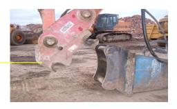
2. Quick Release Hitch being placed on the attachment
