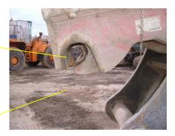
4. Safety Pin is placed into position, this stops the Jaws in No. 3 from being accidentally being released
