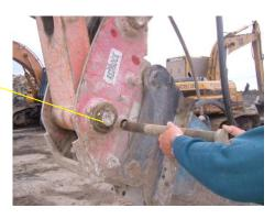
5. Safety Pin in Position with Split Key to keep the Safety
